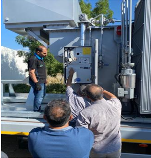
Engineers are testing the tap changer tests (left) and are verifying the specifications and name plate of the substation (right).
